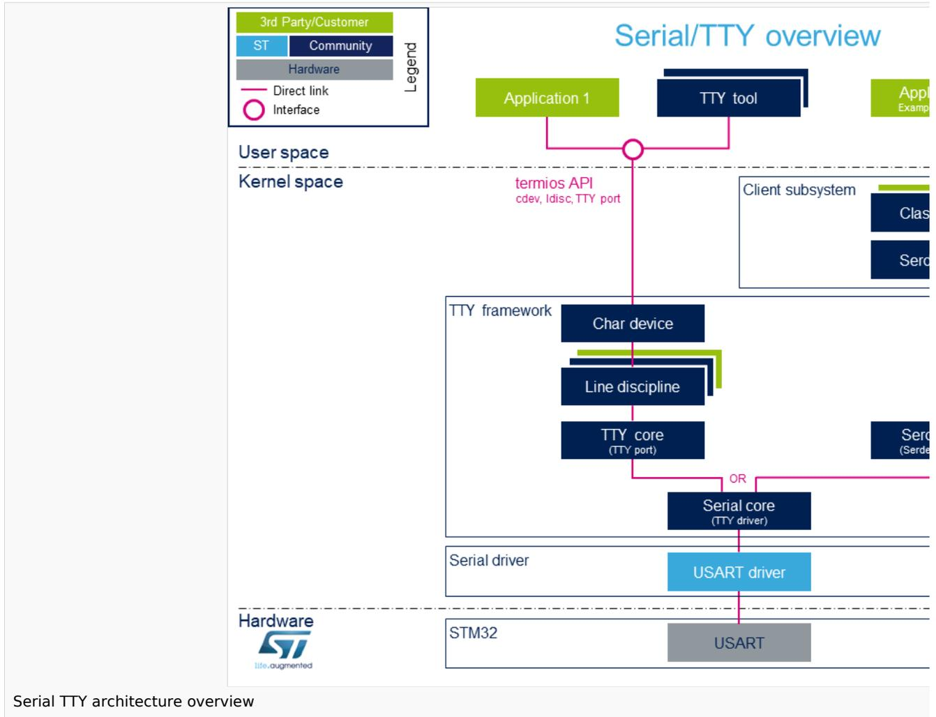
Note: during boot, while a serial device is probed, the serial framework instantiates an associated tty terminal as a virtual device. Then the system sees this tty virtual device as a child of the associated serial device.
