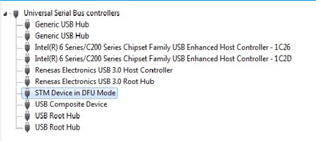
Figure 1: STM32 DFU Device with DfuSe Driver
